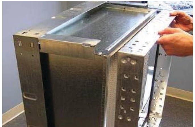
Figure 26: Positioning of the prefilter frame
