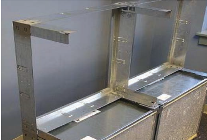
Figure 19: Frame with Leg Extensions Installed
